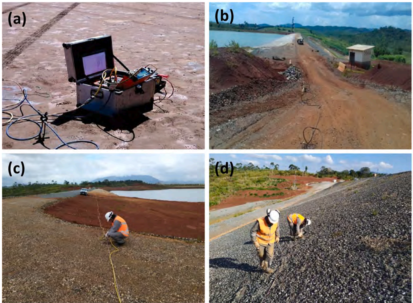
Fig. 3. Photographic record of the ERT campaigns: (a) ABEM SAS4000 resistivimeter, (b)&(c) data acquisition on the crest, and (d) data acquisition on the slope of the embankment.
